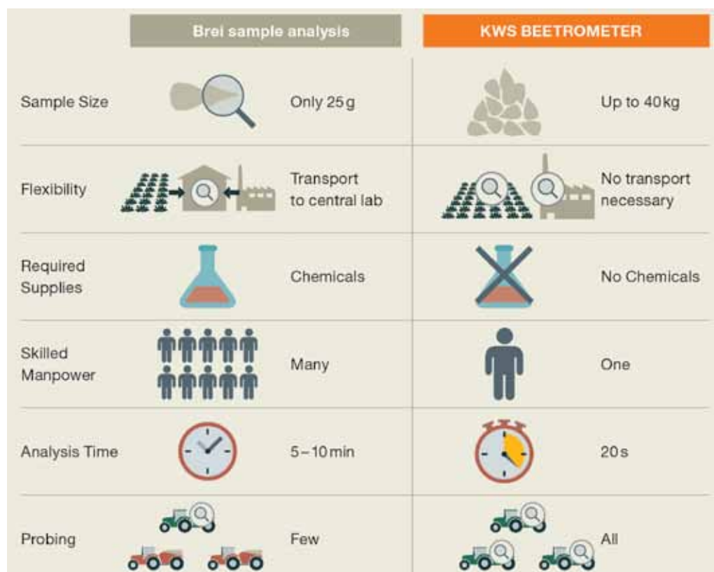
Fig. 2: Overview of requirements for conventional sugar beet brei analyses and benefits of the KWS BEETROMETER
